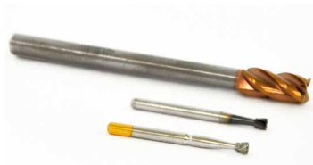
Figure 2 : (from top to bottom) endmill 4 mm diameter, endmill 1.8 mm diameter and an abrasive diamond endmill
