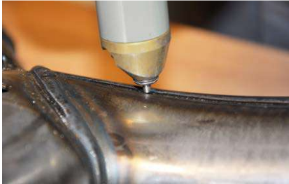
Figure 15 : Ultrasonic needle peening of the weld toe
