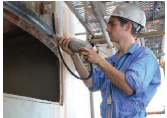
Example of tanker rudder weld peening operation
