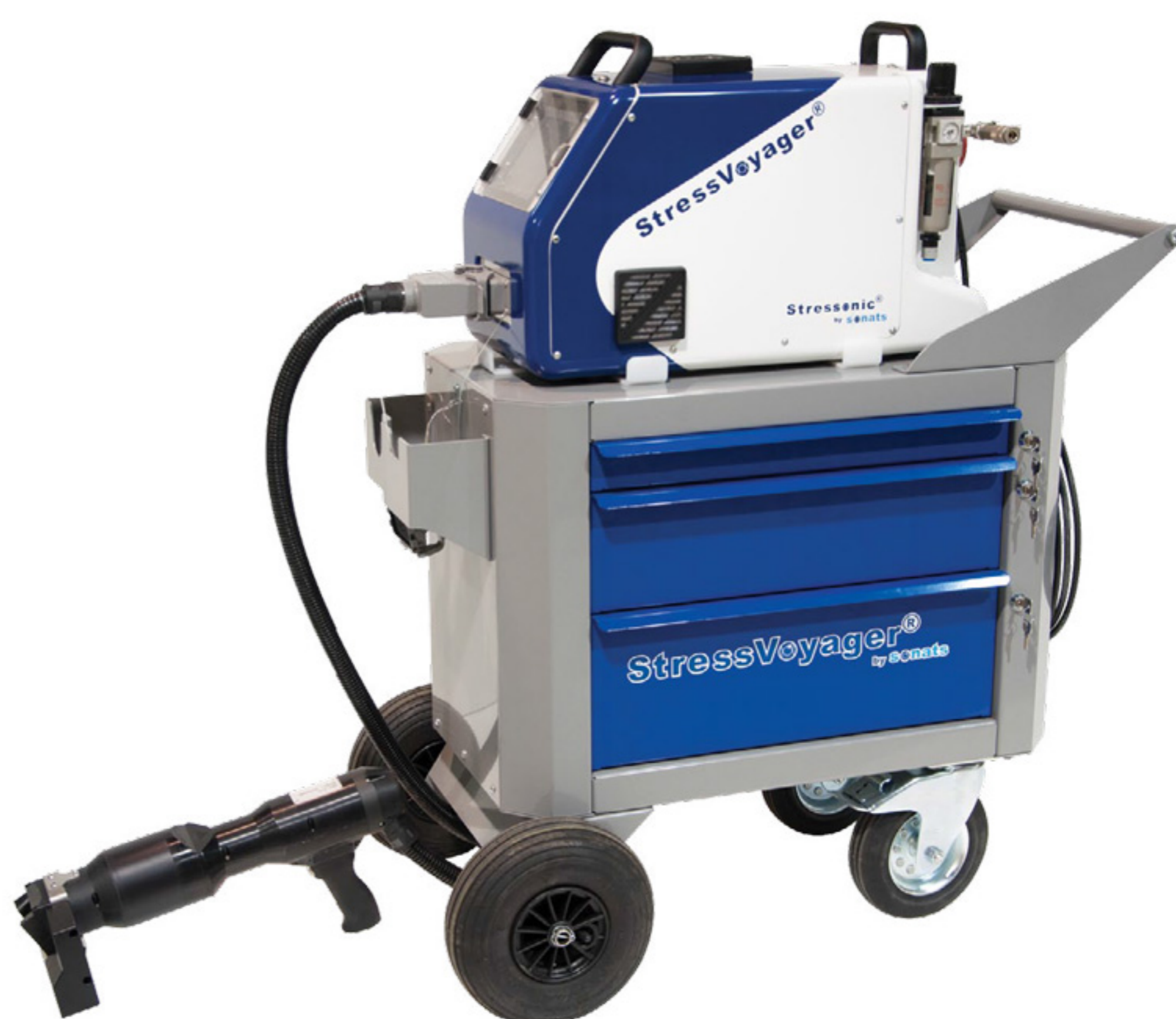
StressVoyager® portable USP equipment on a storage trolley
