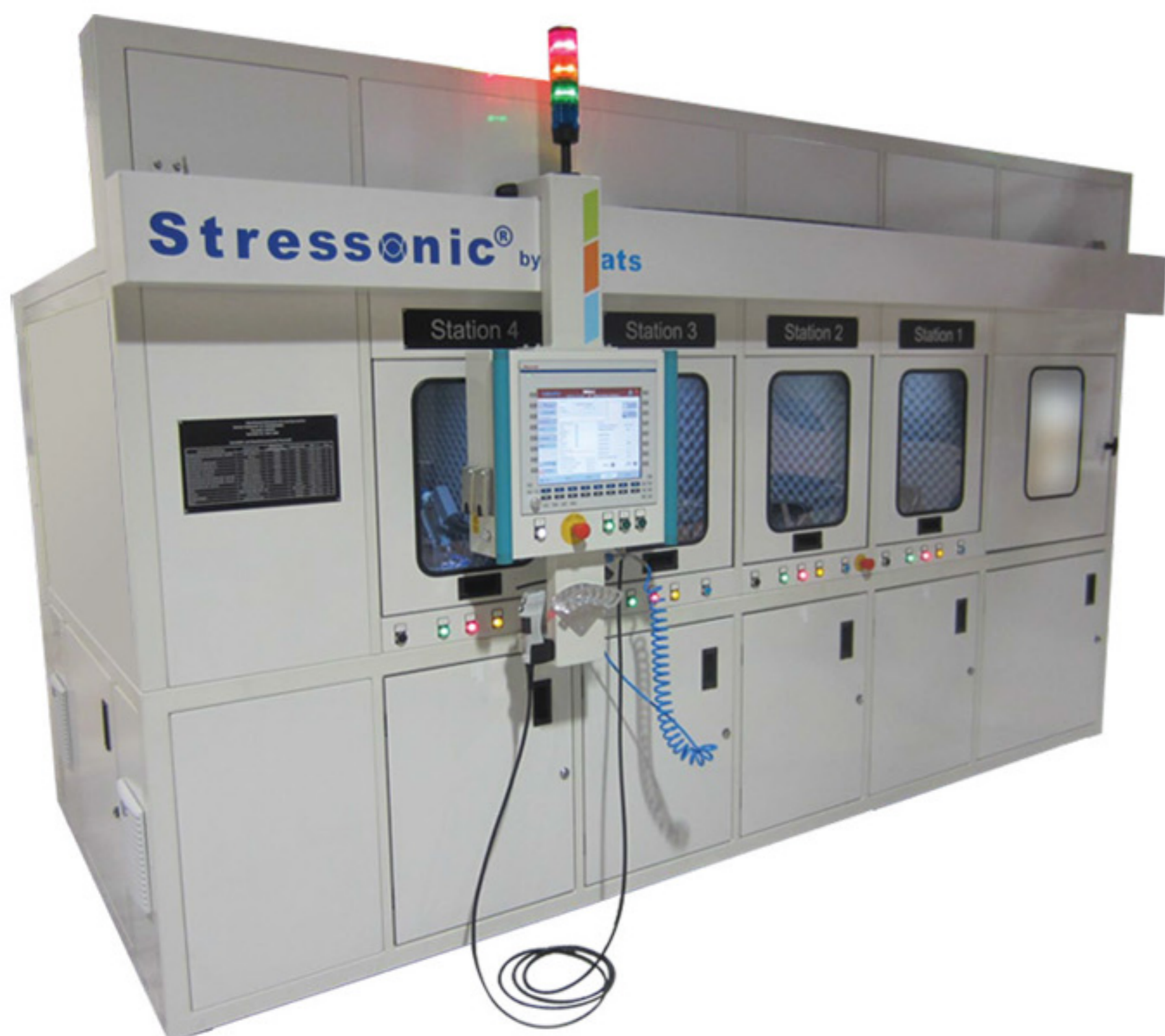
Stressonic®USP automated 4-station machine for automotive output shafts
