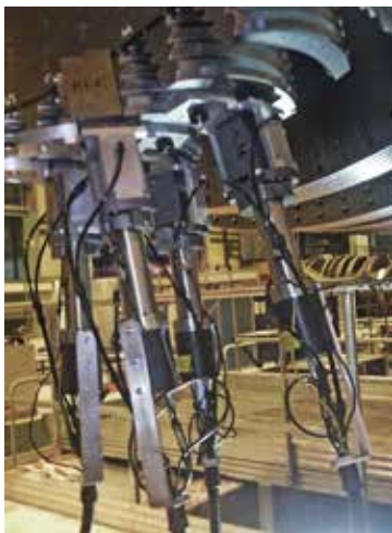
Fir Tree Groove shot peening with portable equipment
