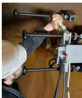
Residual Stress Measurements in situ (NF EN 15305)
